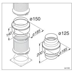
In addition to insulating the exhaust ducting, we recommend that a suitable condensate trap is also installed to collect and evaporate any condensate which may occur. Condensate traps are available for Ø 125 mm or Ø 150 mm ducting.
